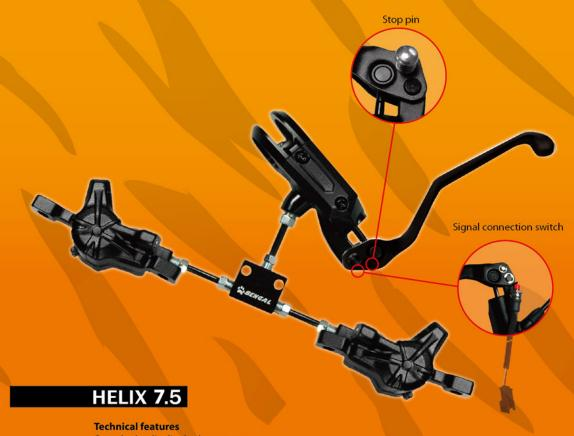
Open hydraulic disc brake system
